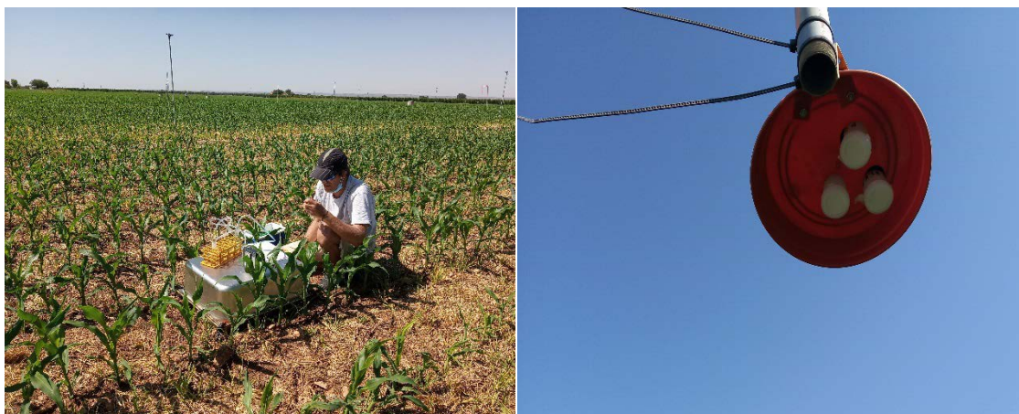
Figure 13. Static hoods and passive \text{NH}_3 samplers for emission monitoring
