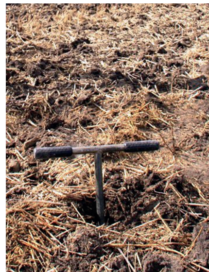
Figure 3: Comparison of the depth of soils in two very different cases. In the image on the left, the effective depth of the soil is limited to a few centimetres due to the presence of rock near the surface. In the image on the right, the auger penetrates to a depth of 100 cm in a clayey soil. The difference in the behaviour and potential of the root system of plants will be very great. Author: M. Aran.
