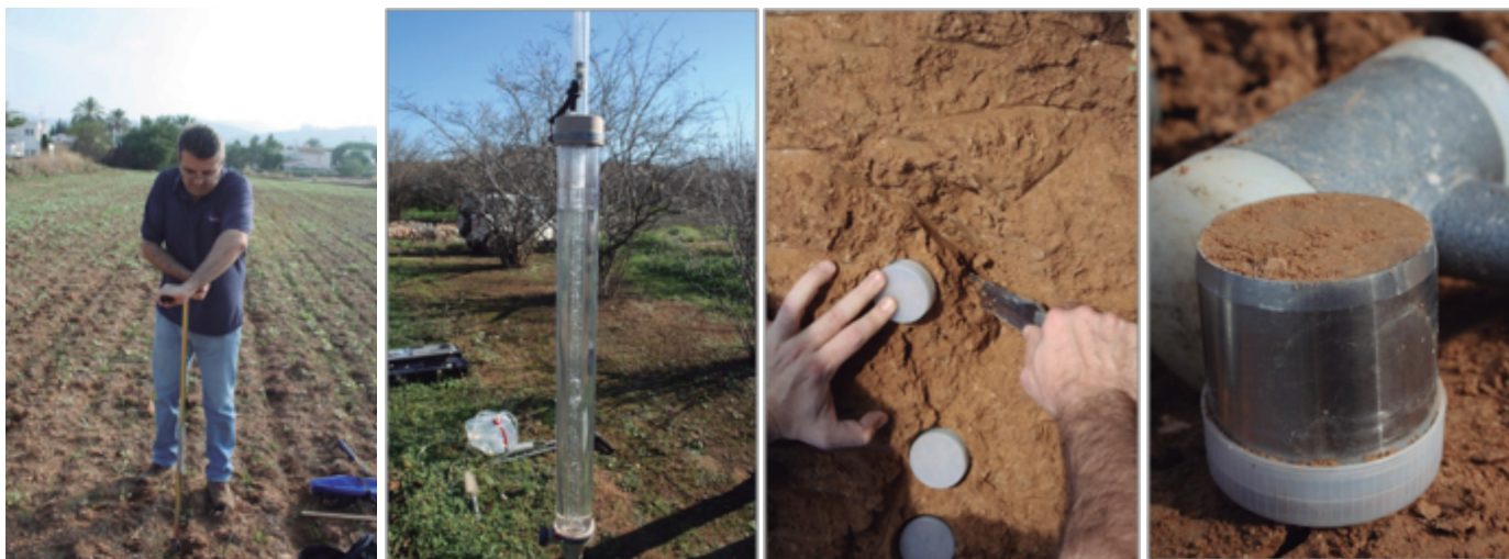
Figure 3: Some complementary determinations for soil characterisation: hydraulic conductivity using a Guelph permeameter, and determination of the bulk densities of a horizon.
